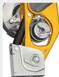
The patented SAF SAFEGUARD-DESIGN of the functional suspension arm reliably protects the brake cylinder from damage.
