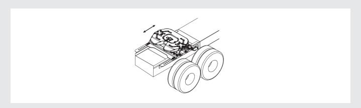
The fifth wheel can be moved forwards or backwards to accommodate different trailer lengths and/or alter weight distribution on the tractor unit.
