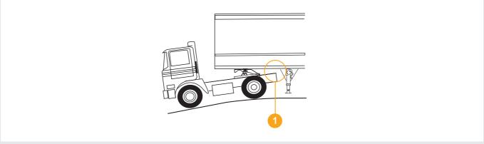
1 Reduced clearance between rear of Chassis and Trailer
