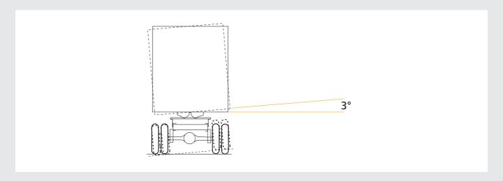
Rotation about the longitudinal axis of up to 3° of movement between the tractor and trailer is permitted. On a standard fifth wheel this occurs as a result of clearance in the fifth wheel to bracket fit, compression of the rubber bushes and also vertical movement between the kingpin and locks may allow some lift of the trailer one side.
